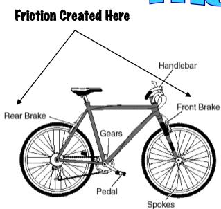
**Friction** is the resistance to motion created by two objects moving against each other. Friction creates heat. The brakes on this bike can create friction to help a bike slow down. **Directions:** In the pictures below, identify if the objects have **potential** energy or **kinetic** energy.
